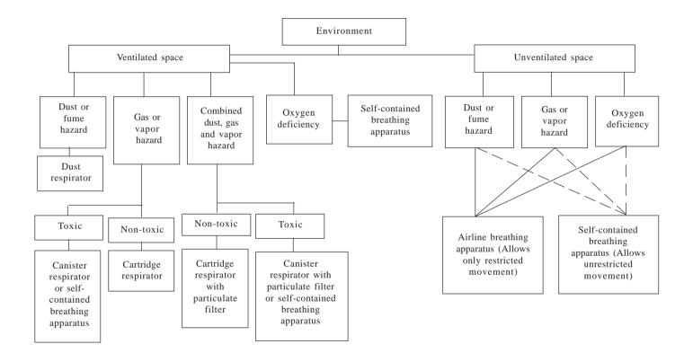
Normally in a ventilated space, oxygen deficiency would not occur, except, due to an accident situation
