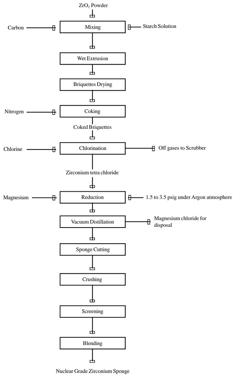
**FIG 6 : PROCESS FLOW SHEET FOR PRODUCTION OF NUCLEAR GRADE ZIRCONIUM SPONGE**
