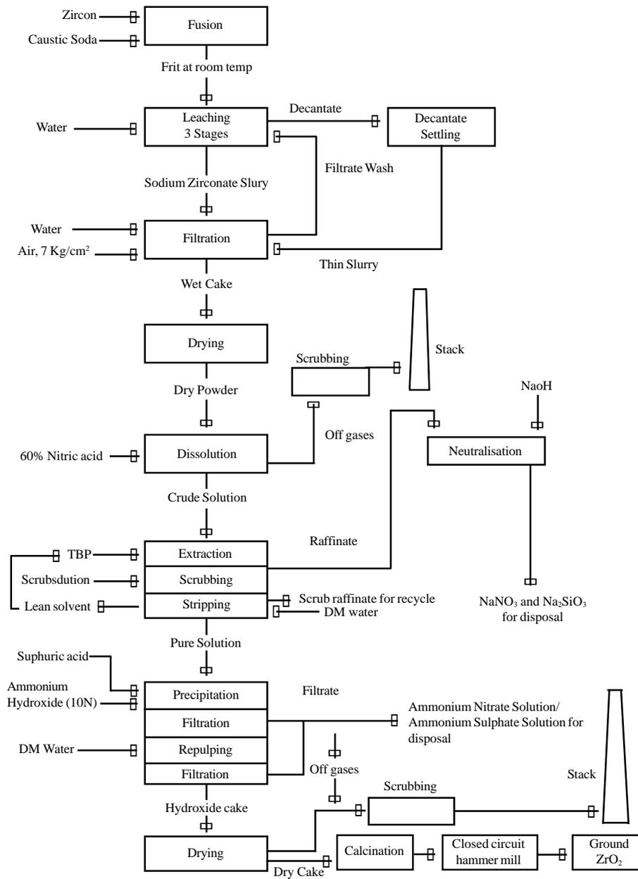
**FIG 5 : PROCESS FLOW SHEET FOR PRODUCTION OF  $ZrO_2$  POWER**
