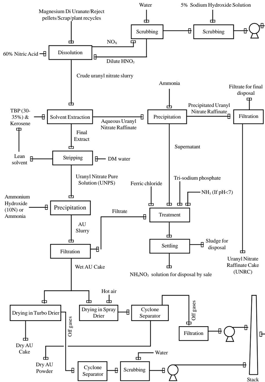
**FIG 1 : PROCESS FLOW SHEET OF WET PROCESS**
