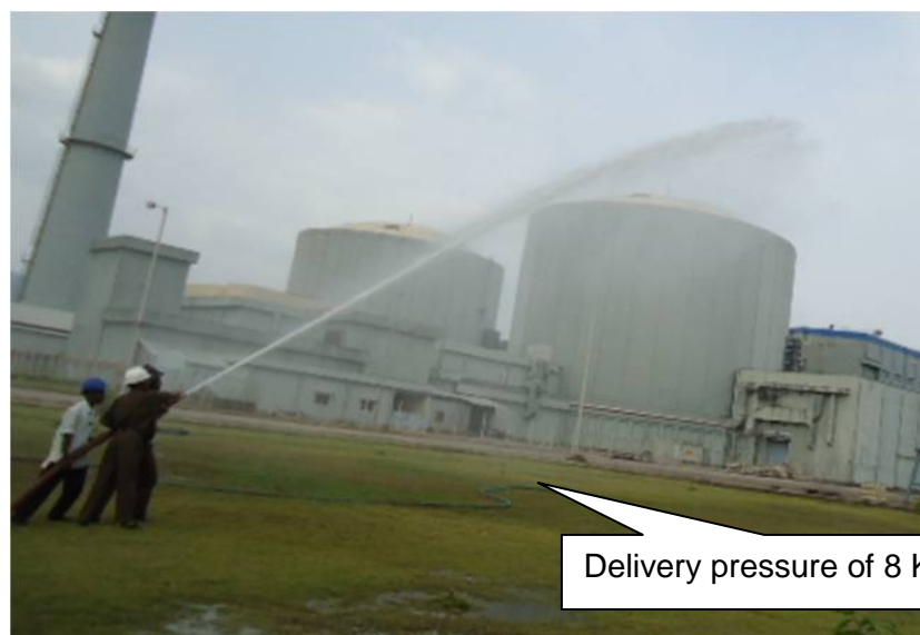
Mock exercise for checking adequacy of mobile pump with the hookup points at KGS-1&2
