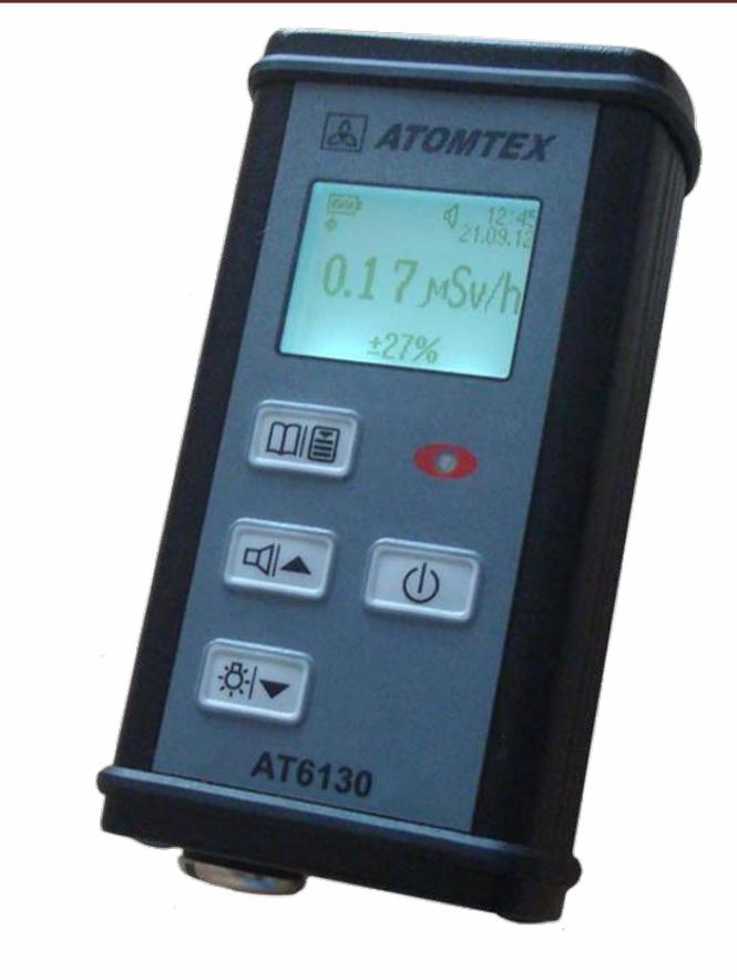
Carry out proper radiation survey while operating radiography equipment
