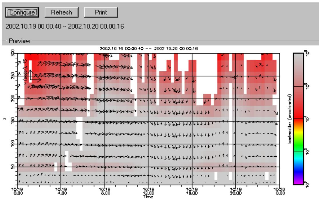
Fig.8 Wind profile for two days . Red patches indicate the mixing layer height
