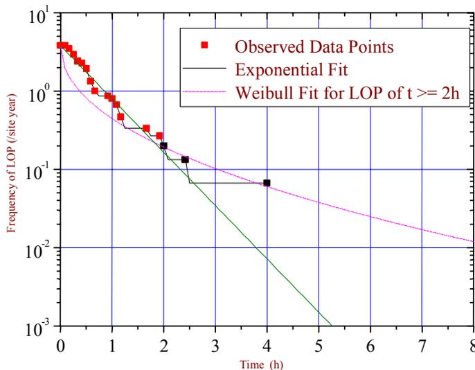
Fig. 2: Frequency of Loss of Offsite Power Exceeding Specified Duration
