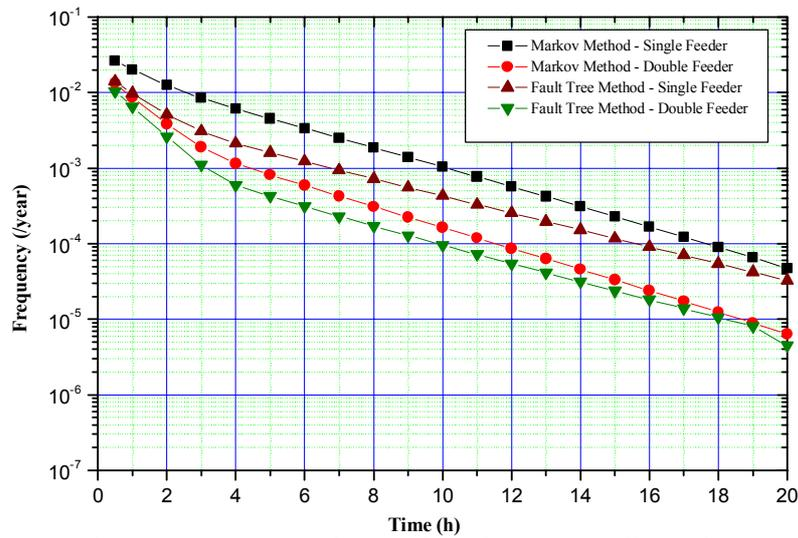
Fig. 5: Frequency of SBO for Time Exceeding Time t
