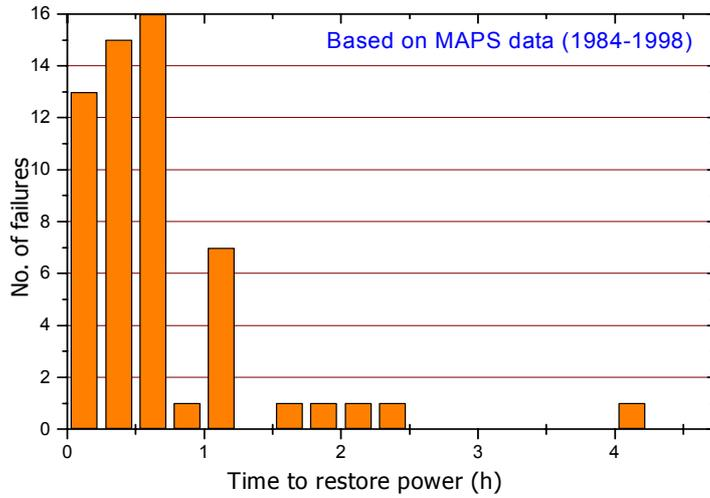
Fig. 1: Frequency Distribution of Failure Duration
