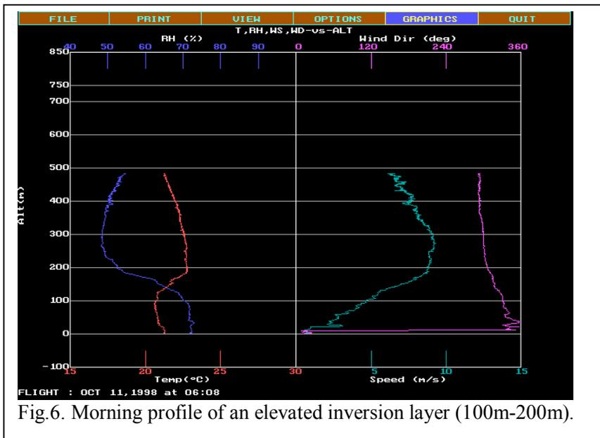
Fig.6. Morning profile of an elevated inversion layer (100m-200m).
