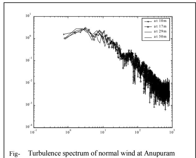
Fig- Turbulence spectrum of normal wind at Anupuram
