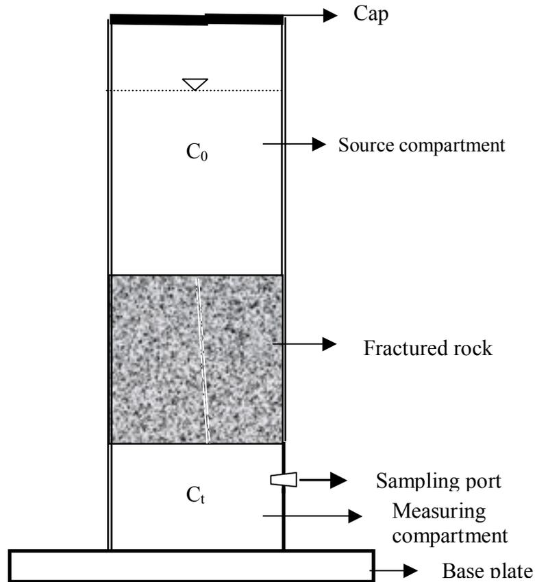
**Fig. 3 Type-II Diffusion cell for testing fractured rock sample**
