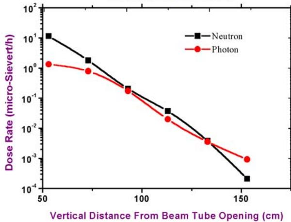
**Fig. 6b. MCNP Calculated Dose Rates on top of the Mobile Shield**
