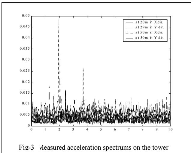
Fig-3 Measured acceleration spectrums on the tower
