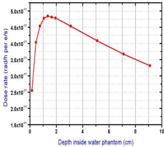
Computed Dose Build up inside Water Phantom for 6MV Beam
