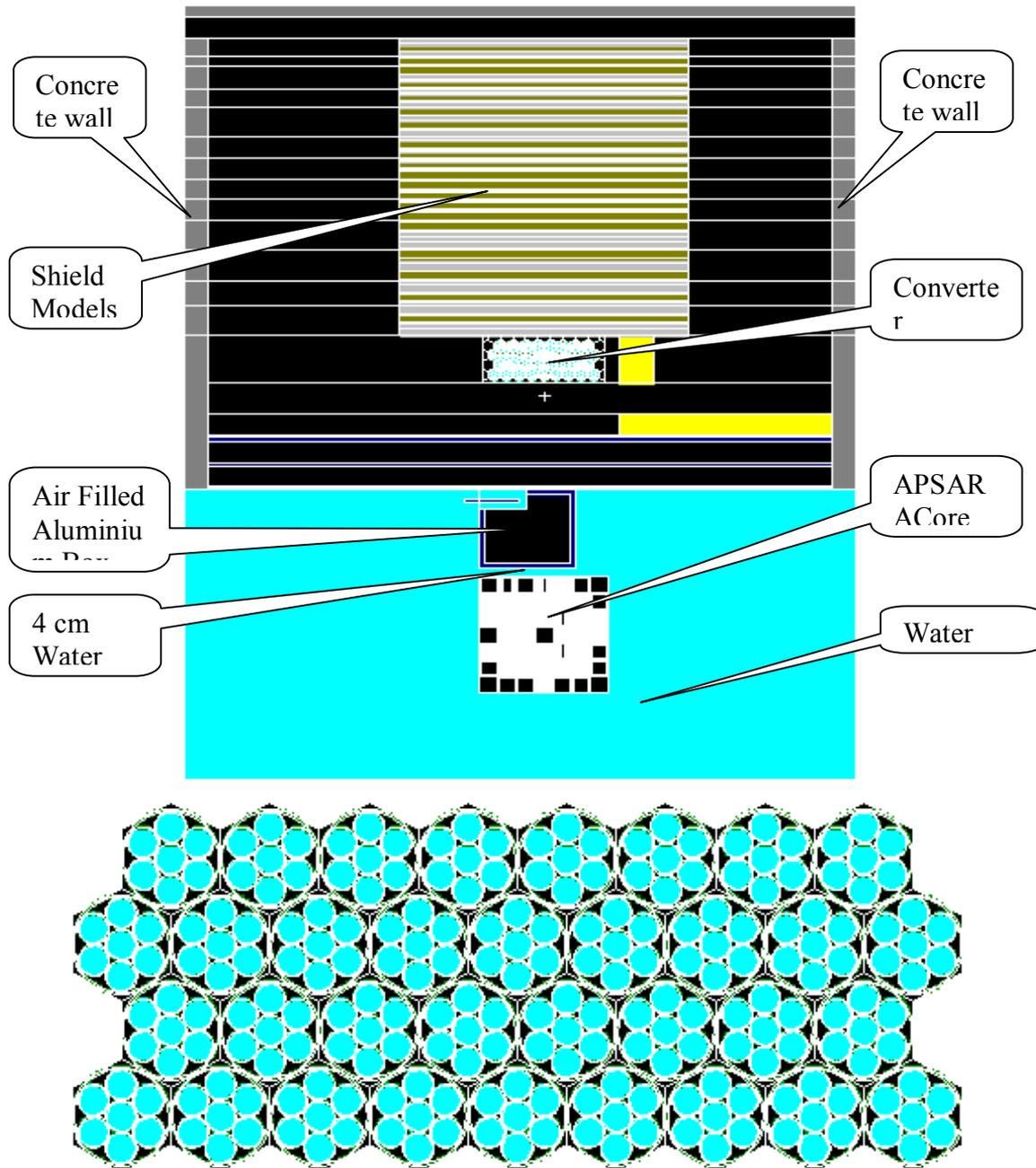
Fig.1 2D MCNP Plot of the Geometry Model of a Typical Experimental SET
