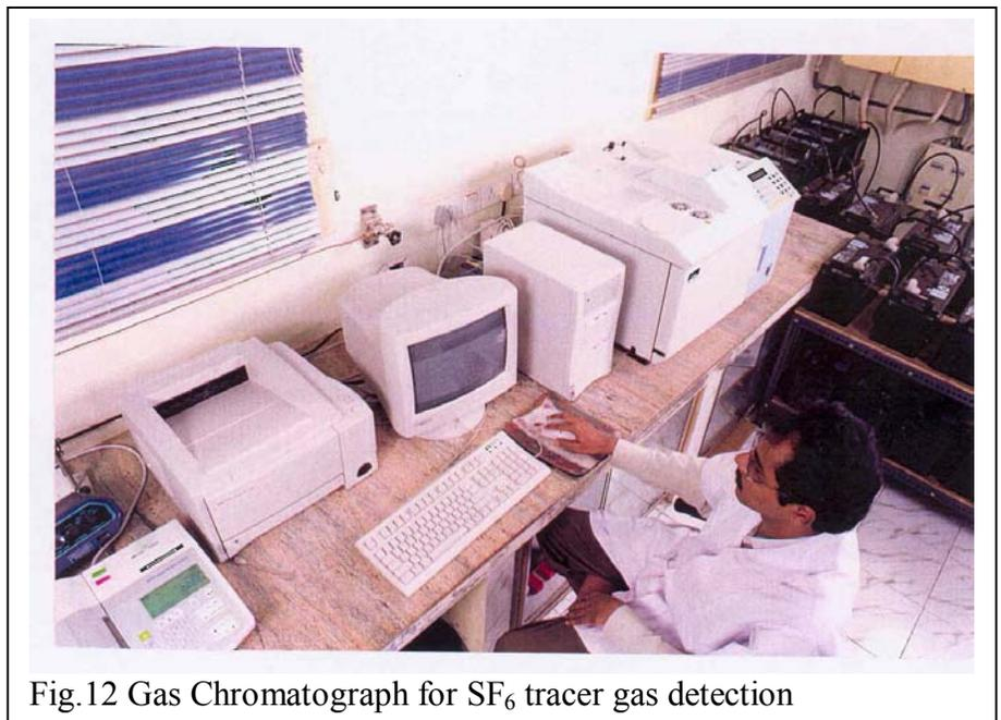
Fig.12 Gas Chromatograph for SF<sub>6</sub> tracer gas detection
