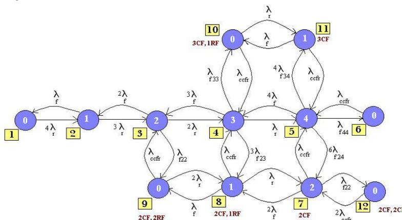
Fig. 3: Markov State Transition Diagram of 2/4 DG Configuration
