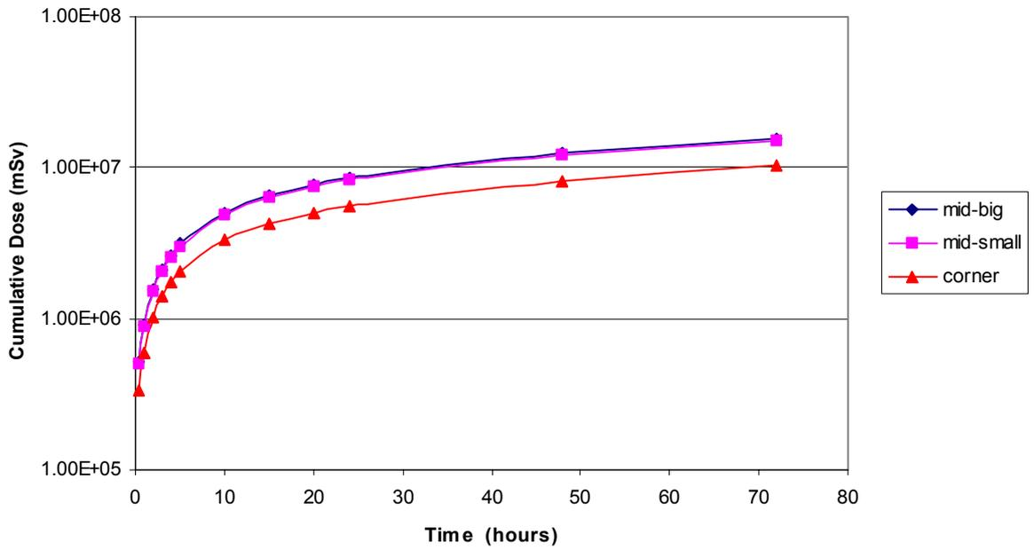
Fig.9: Variation of Dose Rate in Control Room at Different Distances from the RCB Wall after Hypothetical Core Disruptive Accident (EFR Release Fraction)
