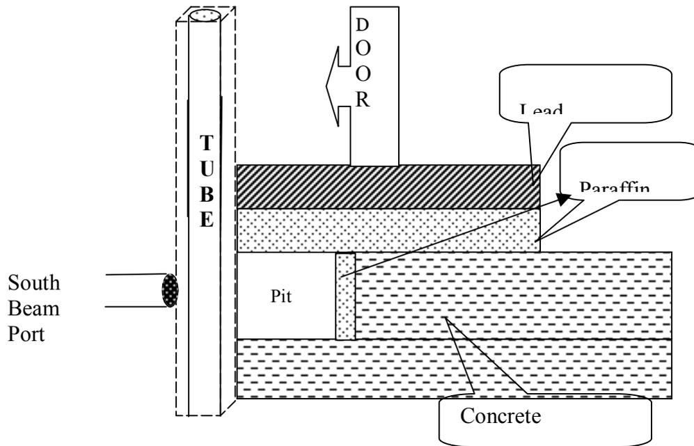
**Fig.4: Elevation view of proposed shielding structure at the south beam**
