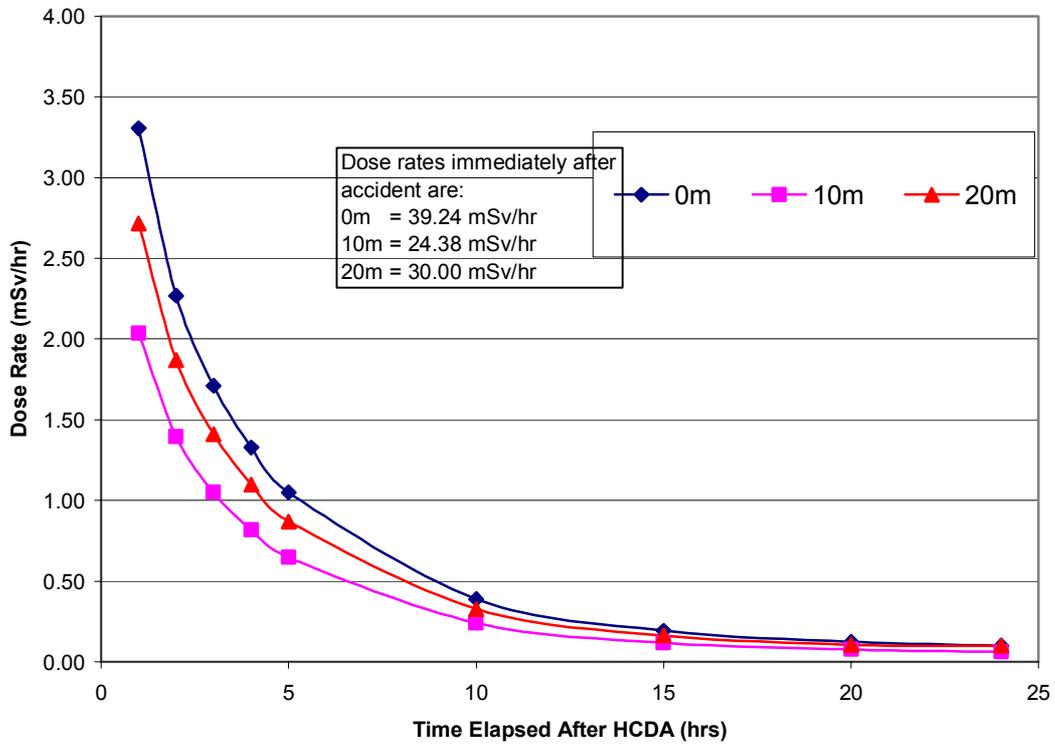
**Fig.10: Variation of Cumulative Dose in Control Room at Different Distances from the RCB Wall after Hypothetical Core Disruptive Accident (EFR Release Fraction)**
