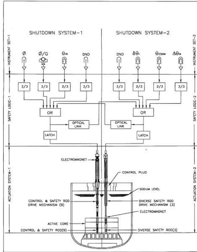
Fig. 6: Shut Down System of PFBR
