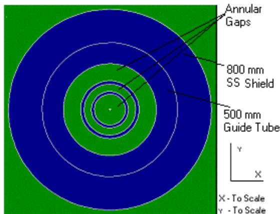
**Fig.7: 2D View of Transfer Arm as Modeled in MCNP Code for Reactor Operation**
