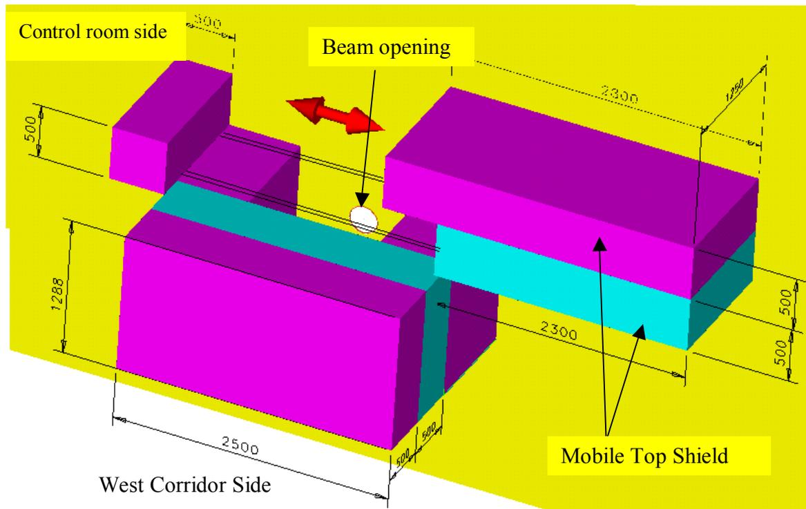
**Fig.5: Isometric View of the Proposed Shield Structure around the West Beam Port**
