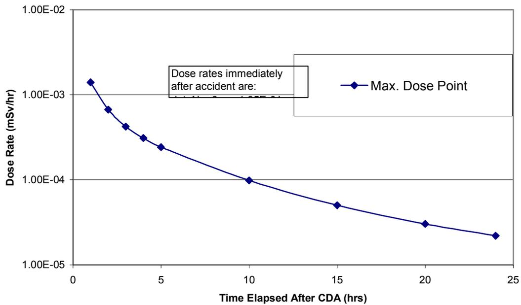
**Fig.12: Variation of Cumulative Dose in Backup Control Room after CDA (OECD Release Fractions)**
