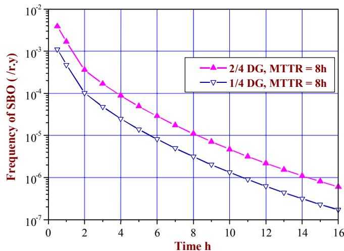
Fig. 4: Frequency of Station Blackout Events Exceeding Specified Duration
