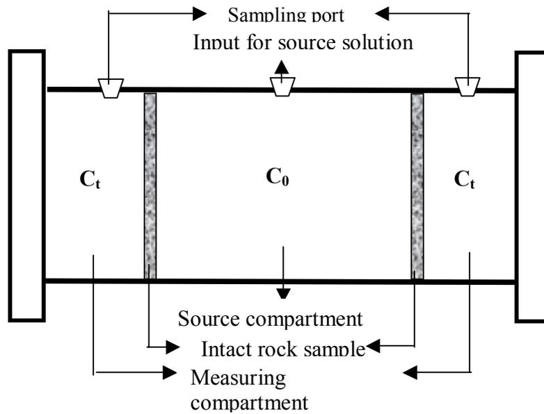
**Fig. 2 Type-I Diffusion cell for testing intact rock samples**
