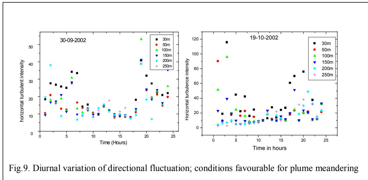
Fig.9. Diurnal variation of directional fluctuation; conditions favourable for plume meandering fluctuation is large during transition times when the wind speed is very low. The  $\sigma_\theta$  is values are shown in Fig.9.
