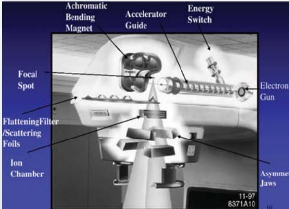
Fig.14A: Schematic of LINAC Head with Beam Flatteners
