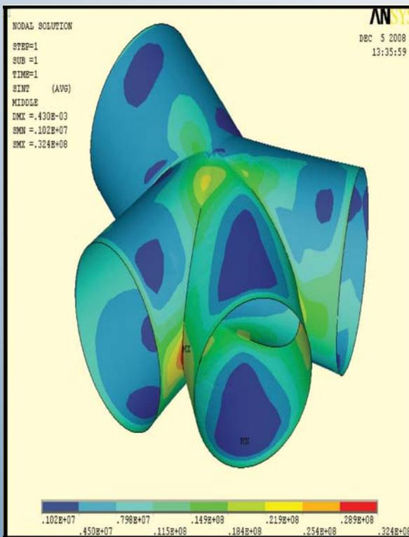
Fig.4 Membrane stress intensity in the branch
