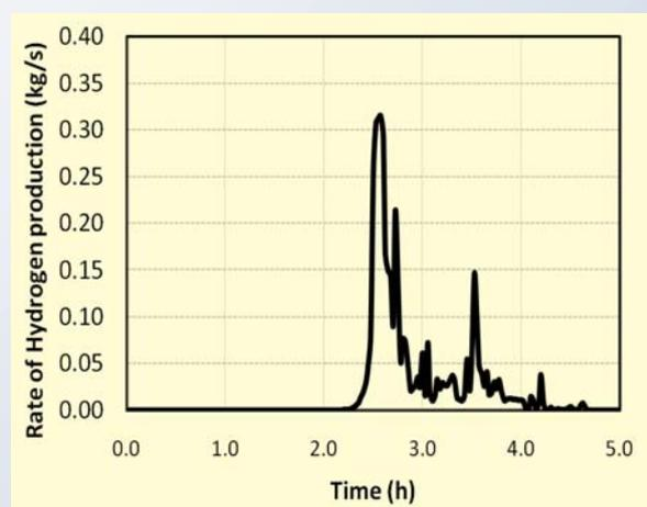
Fig.3 Hydrogen generation with time (ASTEC result)
