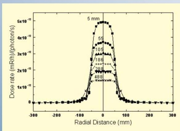
Fig. 10: Calculated dose rates above the exit of the pit. Height from the top of pit is indicated in mm (work carried out in collaboration with IGCAR)
