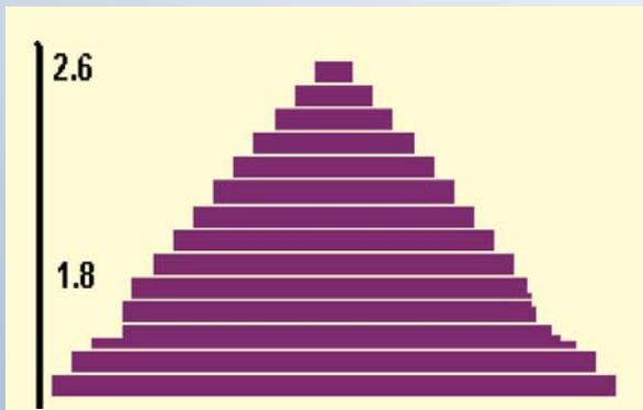
Fig.15: Approximate shape of beam flattener
