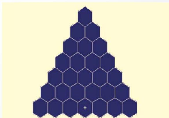
Fig.7: Closely stacked lattice of 28 FSA (Triangular shape)
