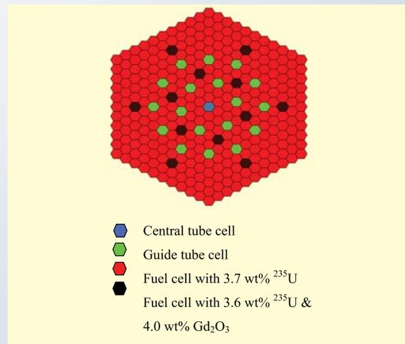
Fig. 3: Schematic diagram of a uniform LEU fuel assembly
