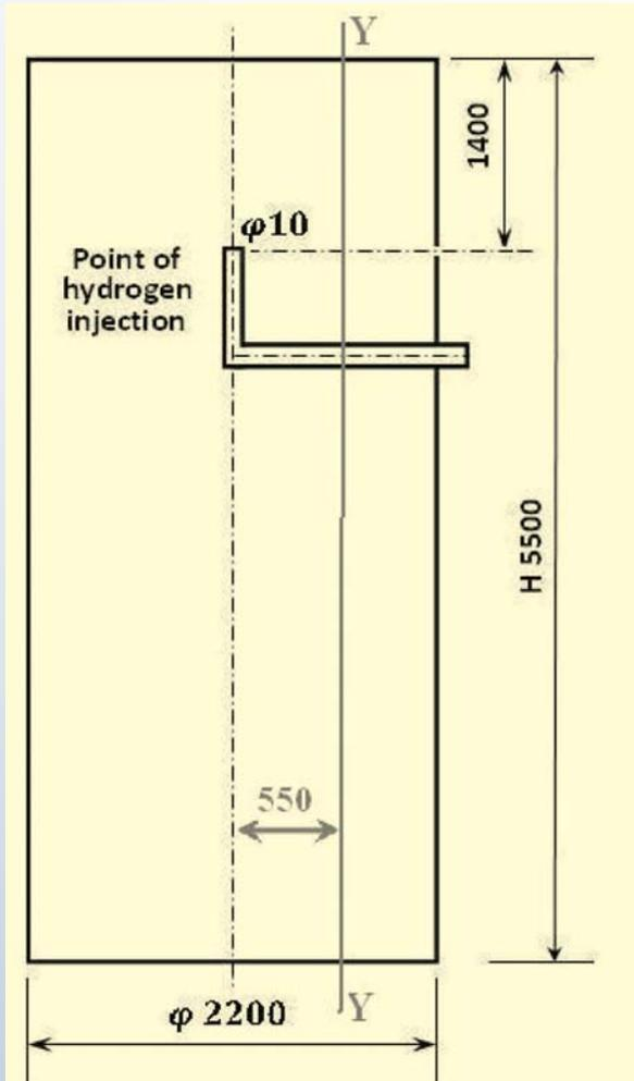
Fig.4 Geometry of setup for hydrogen distribution (dimensions in mm)
