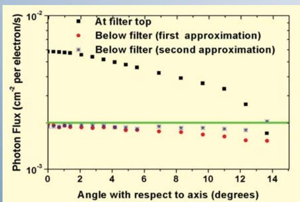
Fig.16: Monte Carlo simulated intensity levels with iterations. Green line is the desired level
