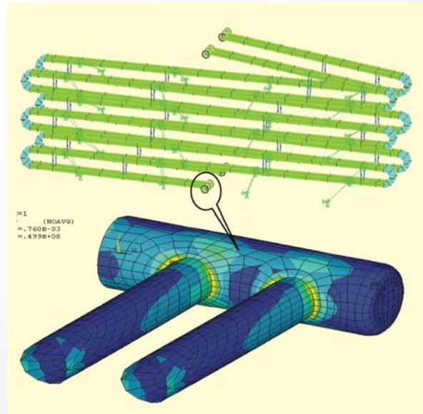
Fig.2 Membrane stress in SG Header of FBTR
