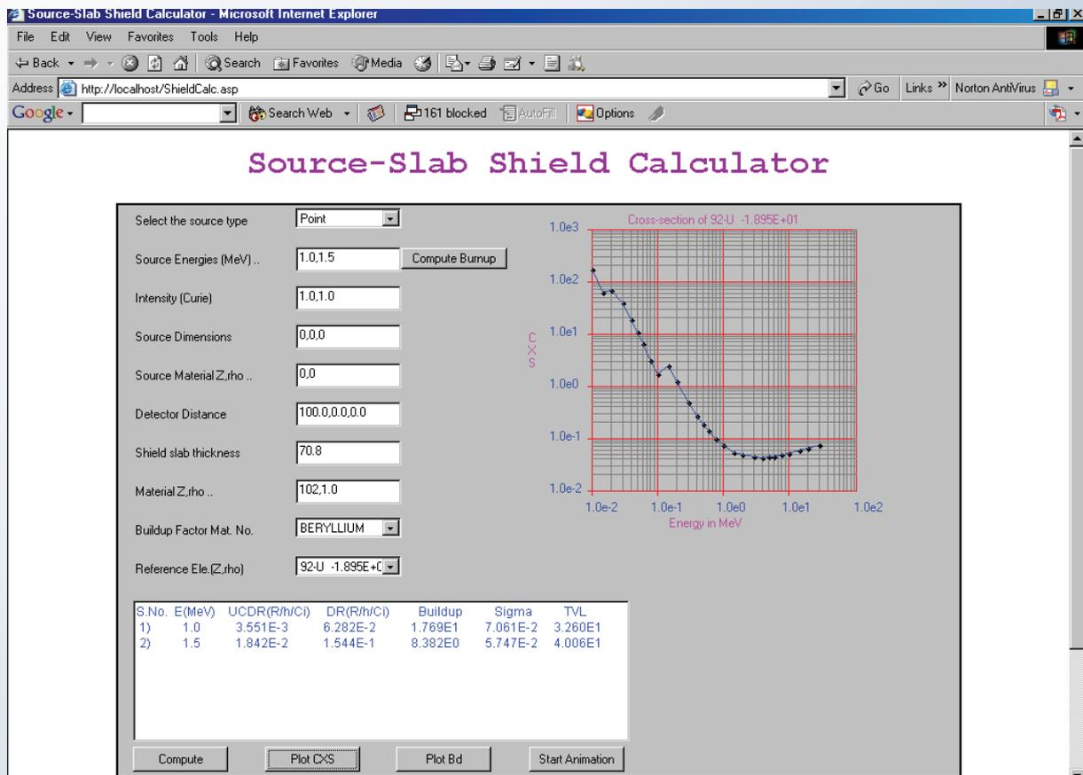
Fig.20: ASP page layout of source-slab shield calculator. On right side display of log-log graph of U-235 photon cross section
