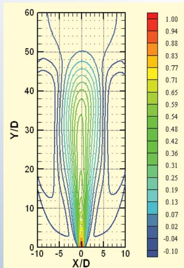
Fig.6 Contour plot for jet of air (Reynolds number of 42).
