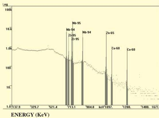
Fig.13: HPGe gamma ray spectrum of irradiated and cooled Garter spring. Prominent isotopes are indicated
