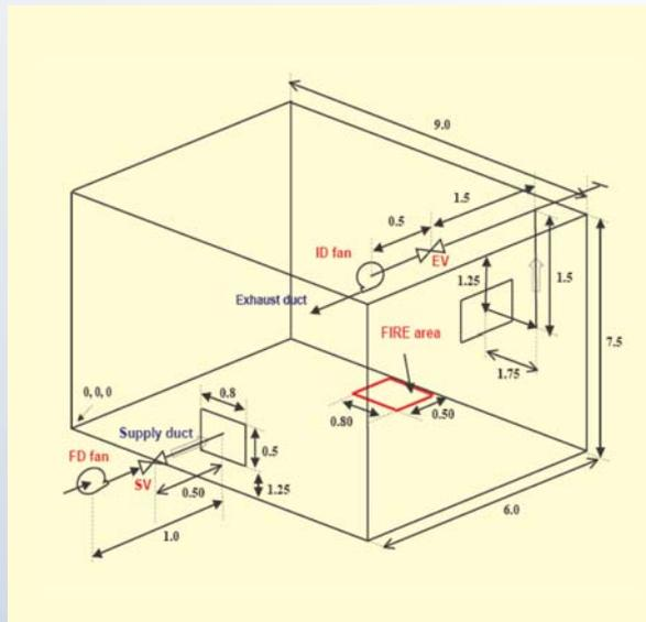
Fig.1 Schematic of the enclosure (dimensions in metres)
