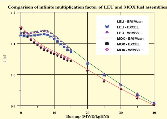
Fig.5: Variation of  $k_{inf}$  with burn up for LEU and MOX fuel assemblies
