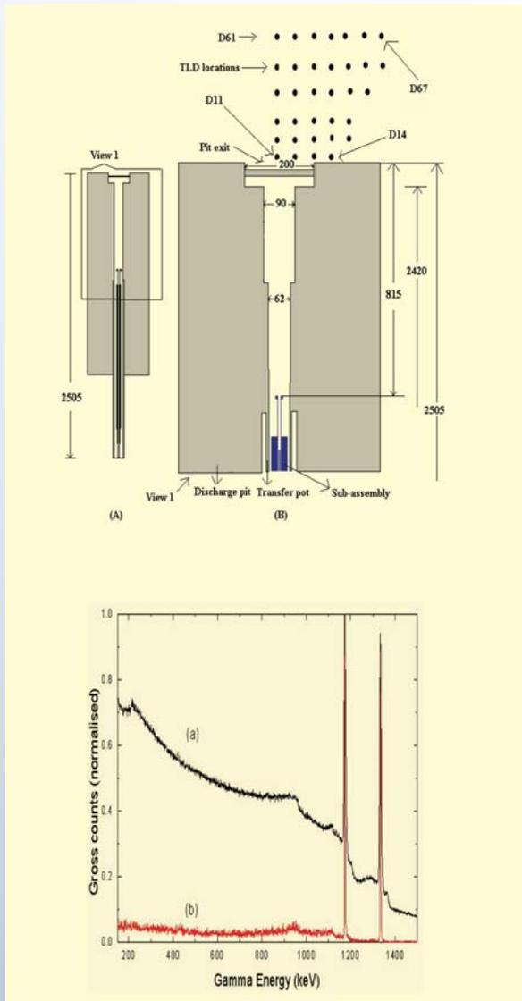
Fig.9 (A): Schematic diagram of subassembly storage pit of FBTR
