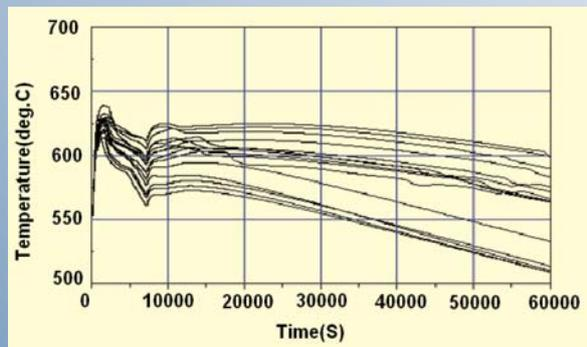
Fig. 3 Evolution of Hot Pool Temperature as function of time when 3 loops failed at 2h.
