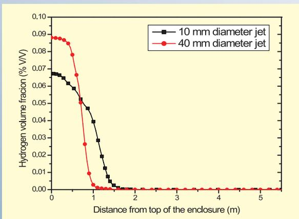
Fig.5 Hydrogen volume fraction vs distance from top of the enclosure
