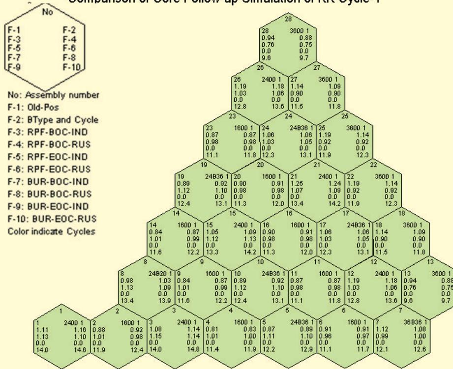
Fig.2A: Comparative study of KKNPP 1/6 symmetric fresh core
