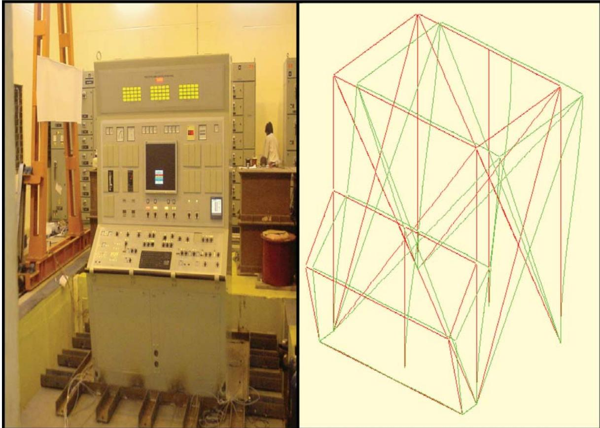
Fig.5 (a) Control Panel (b) Deformed shape of idealized model the under tri-axial excitation
