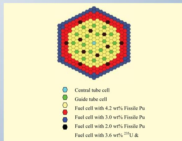
Fig. 4: Schematic diagram of a profiled MOX fuel
