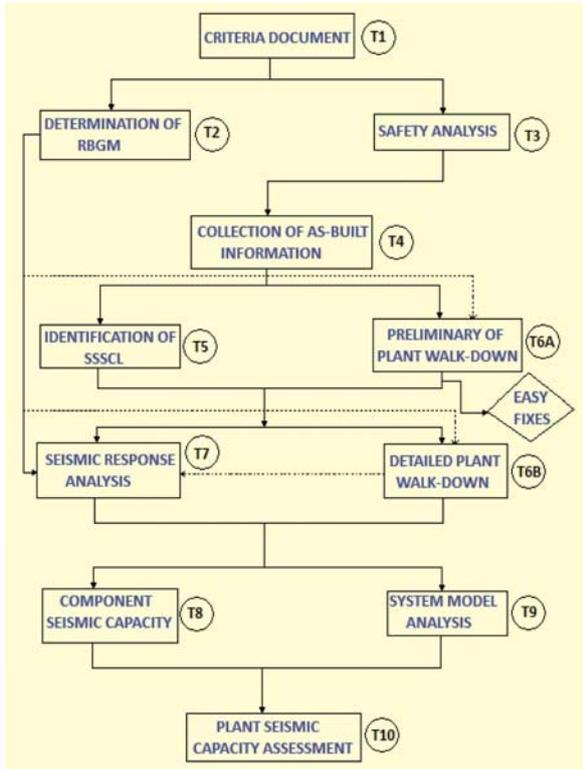
Fig.4 Task flow for seismic re-evaluation of FBTR
