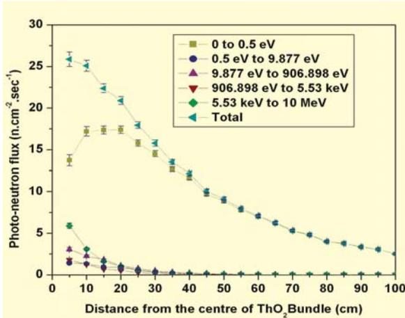
Fig.11: Radial Variation of Photo Neutron Flux in D<sub>2</sub>O Pool
