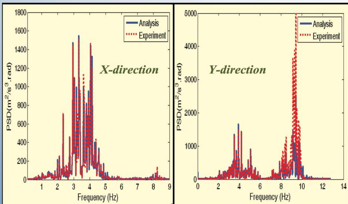
Fig.7 PSD of Response (acceleration) of panel from Experiment and Analysis
