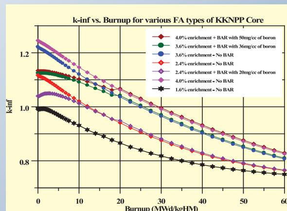
Fig.1: k-inf vs. burn up for various FAs of KKNPP core
