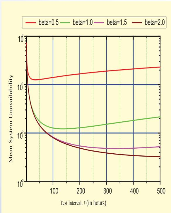
Fig.6 Mean System Unavailability with Weibull Failure Time distribution for 1/2 DG configuration
