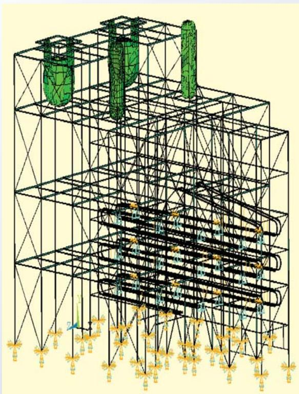
Fig.1 FEM model of SG, Expn.Tank and Surge Tank along with the steel structure
