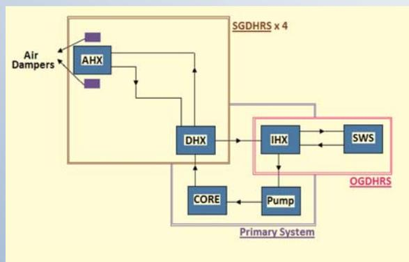
Fig.2 Reliability block diagram of DHR of PFBR.
