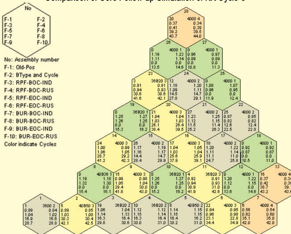
Fig.2B: Comparative study of KKNPP 1/6 symmetric core for 8<sup>th</sup> cycle results. Different colors indicate the number of cycles faced by the FAs.
