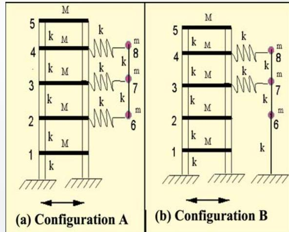
Fig.9 Configuration of system analysed for Multiple Support Excitation
