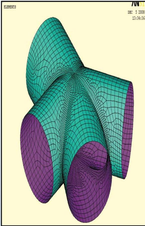
Fig.3 FEM model of a branch connection
