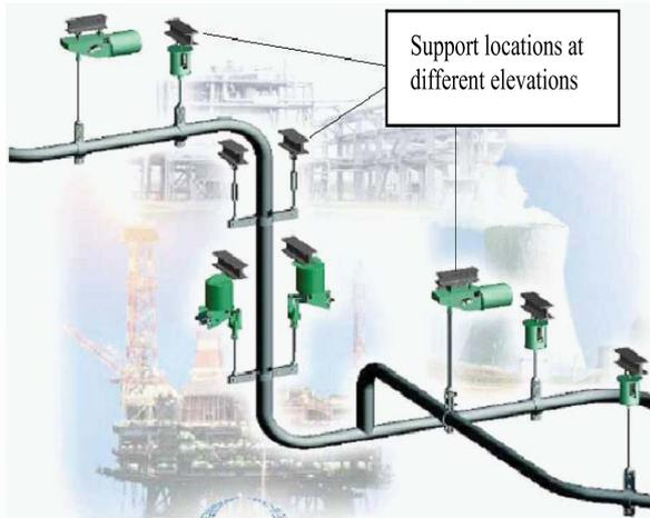
Fig. 8 A typical pipeline supported at different elevation
