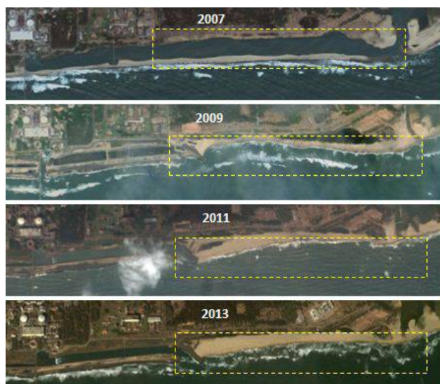
Fig. 8 : Disappearance/disuse of old canal due to construction of new canal at the northern end of the canal
