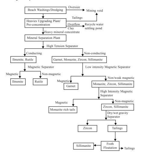
FIG.1: TYPICAL FLOW CHART SHOWING SEPARATION OF HEAVY MINERALS
